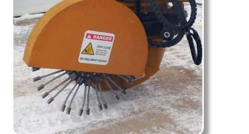
The Cold Air Blower has a Flanger attachment that will help clear out buildup of ice.
