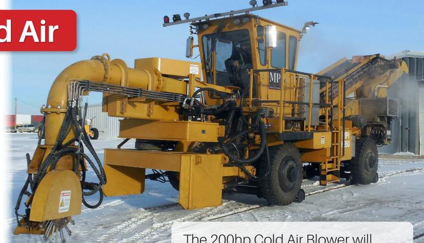
The 200hp Cold Air Blower will produce 9,500 cfm of air with a 275 miles per hour air speed discharge.
