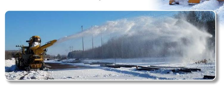
The 200hp Snow Blower can cast snow up to 150 feet away, weather depending.
